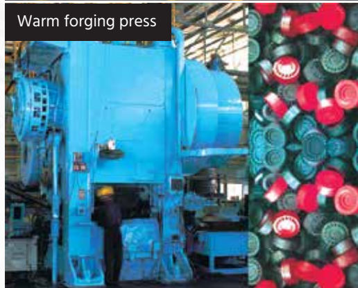
1600 Ton fully automated hot forging press from Kurimoto, Japan
