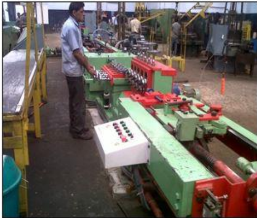
Combined Drawing Machine for Hexagonal / Sections ranging from 5MM to 14MM
