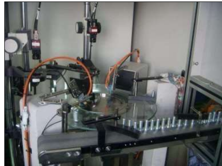
Inspection with Automatic Optical Sorting Machine
