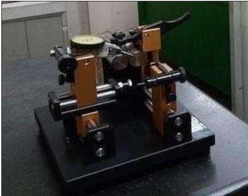
The Standard Room equipped with the Contour Tracer and Concentricity Gauge
