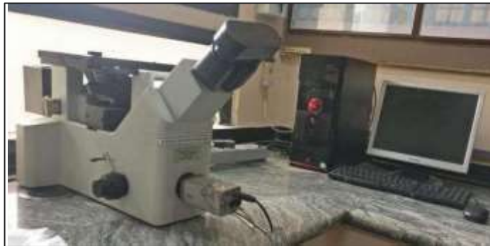
The laboratory equipped with the Coating Thickness Tester and Metallurgical Microscope
