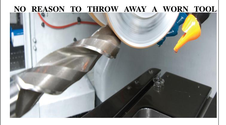
Brancs Reconditioning Program offers more than just basic re-grinding of tools. This service provides "as new" performance at a recondition price cutters are re-manufactured using the original equipment, programs and coating, by the same experienced staff that provided the original tool.
