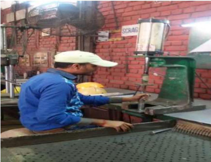
SCRAGGING OPERATION WITH SINGLE SPRING PRESS
