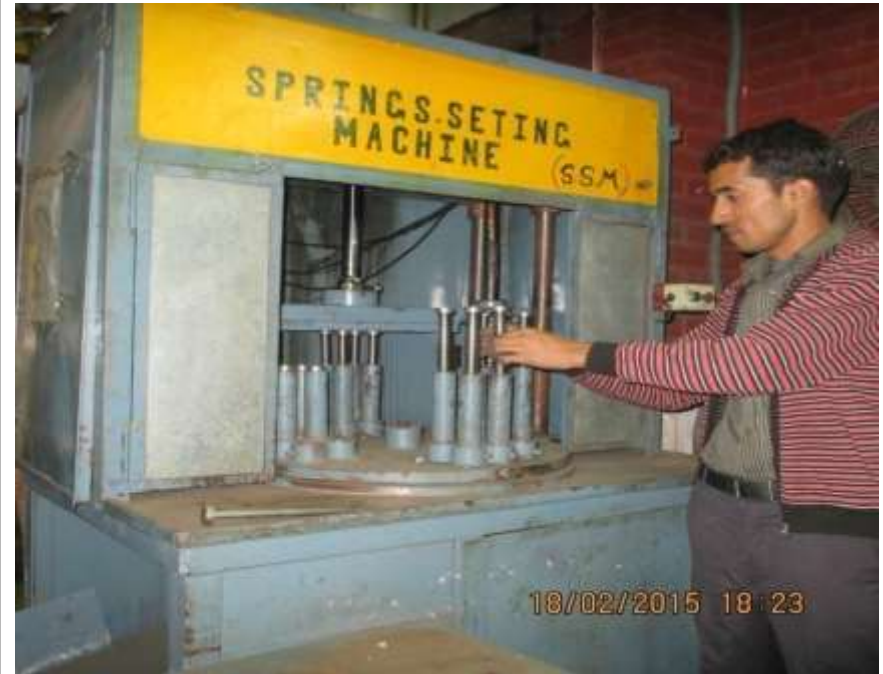
SCRAGGING ACTION WITH FOUR SPRINGS IN ONE OPERATION
