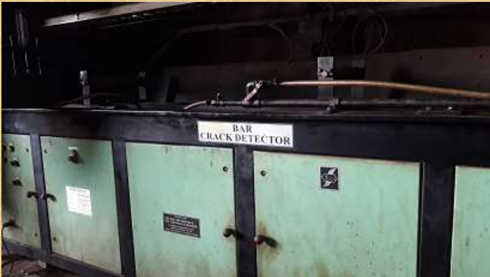
MPI testing for surface and sub surface crack Detect
