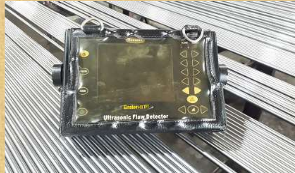
Ultrasonic Testing Machine to find out Internal Crack
