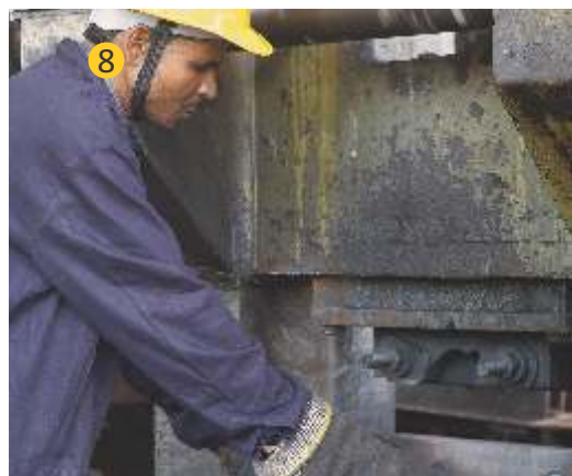
Cutting: The rolled products are sized to batch and order
