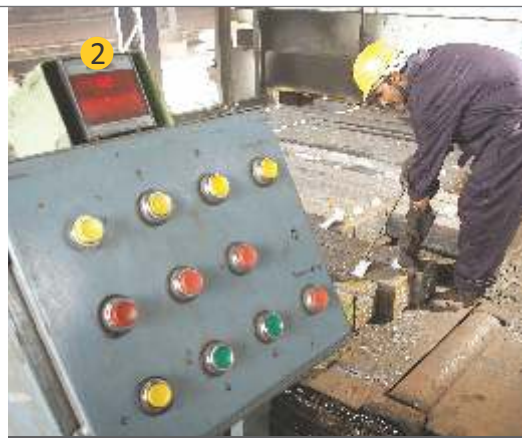
Counter & Pusher: Batched ingot or billets are pushed into furnace
