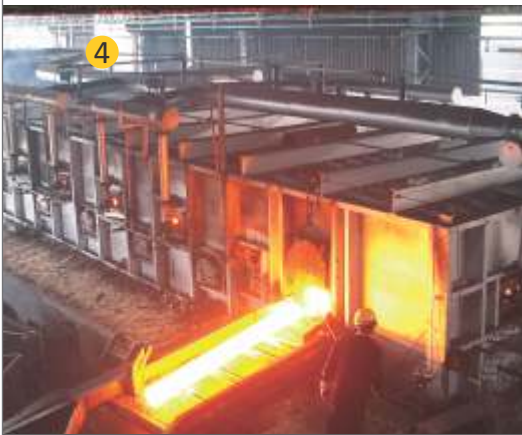
Ejector: Hot raw material from the furnace ready for rolling
