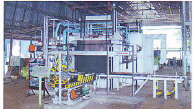
Continuous Pusher type Hardening, Tempering and isothermal annealing Furnace.
