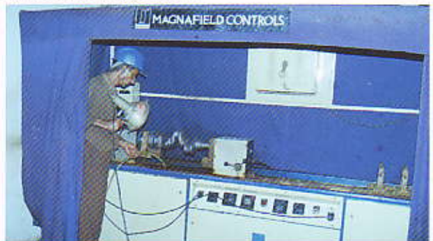
Magna-flux Crack Detection Machine.
