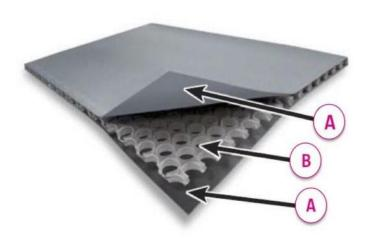
In the industrial process the honeycomb structure is the basis for Sandwich Panel's formation, where A are skins or faces and B the honeycomb core.
