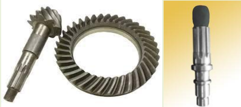
Figure Showing Sample Pasted with Anti-Carburizing Compound
