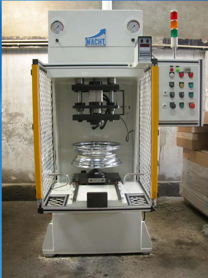
2 Stage Automatic Hydraulic Press for Bearing Pressing & Pre- loading Customer : Harley Davidson
